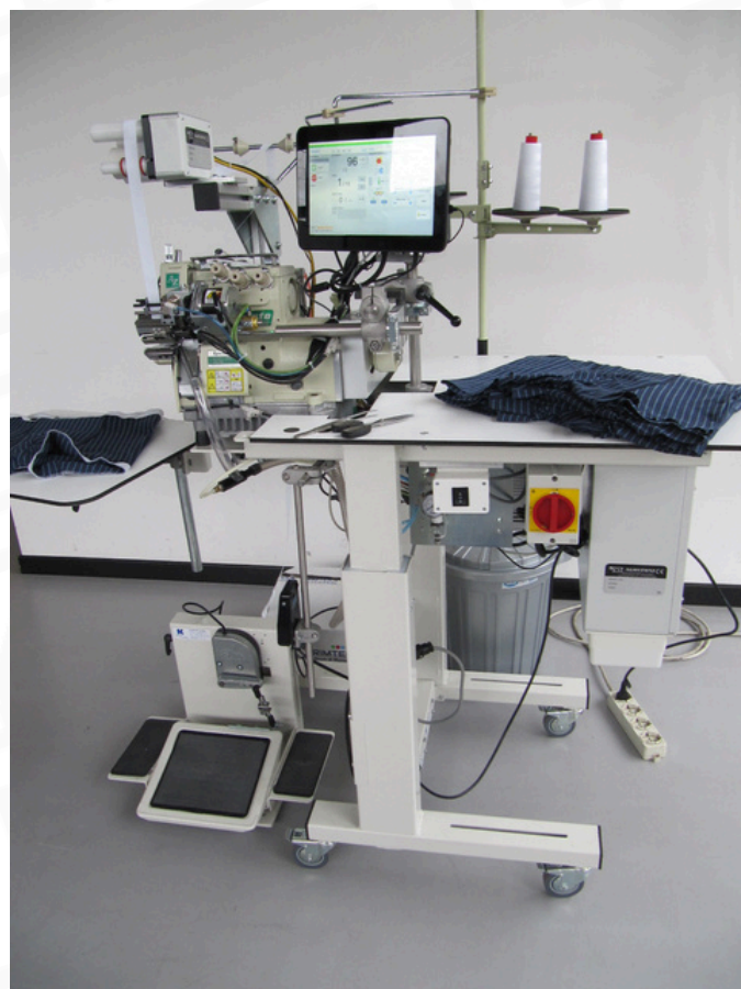
Application example on Overlock Machine with elastic inserter and MiniDigitens for digital tension control
